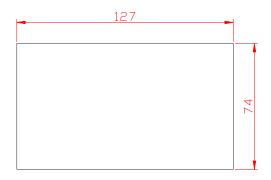
The AIM-T500 insulation monitor adopts embedded installation, and the above diagram is the hole dimensional drawing of the insulation monitor.
