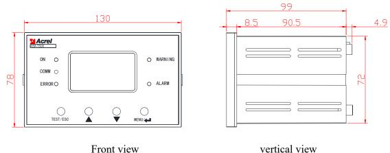
above diagram is the rear view, side view and front view of the AIM T500
